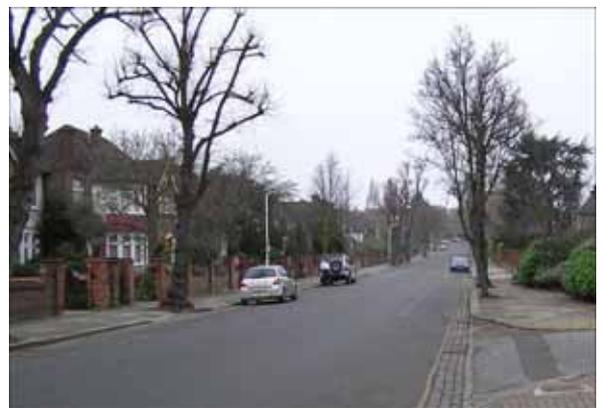
As you can see, many of the roads are quite wide and traffic often exceeds the 30 mph speed limit. The proposal was to have a 20 mph zone over the whole area, to add speed humps to certain roads (they were already present on some) and use speed display devices, mini-roundabouts and "rippleprint" (a proprietary road surface treatment) in other spots.
